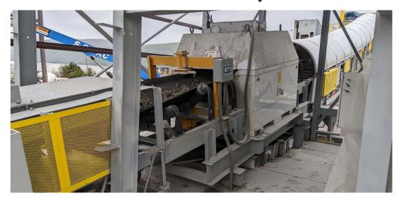
The ETI Model 730-CM is an Online Bulk Material Analyzer utilizing prompt-gamma neutron activation (PGNA) elemental analysis combined with single-gamma density measurement to produce continuous process information. First in its class to directly measure variation of flowrate within the analyzer, it creates best-in-class accuracy.
