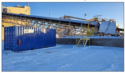
The ETI Model 730 is an Online Bulk Material Analyzer utilizing prompt-gamma neutron activation (PGNA) elemental analysis combined with a Dual-Gamma Ash Analyzer producing ash, moisture, sulfur, & heating value measurements.
