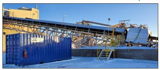
The ETI Model 730 is an Online Bulk Material Analyzer utilizing prompt-gamma neutron activation (PGNA) elemental analysis combined with a Dual-Gamma Ash Analyzer.
